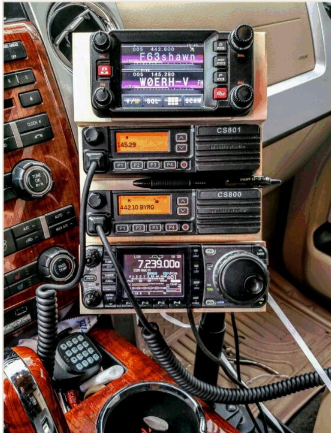
Figure 1: An Amateur Radio Mobile Installation. This is a sophisticated setup that can routinely communicate both locally and nationally, and is ideal for emergency deployment.
