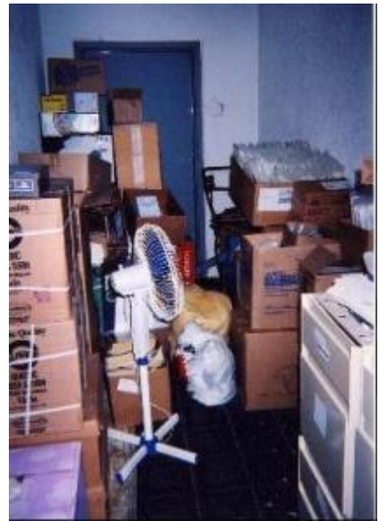
Fire hazard blocked back exit with lawn mower as a “back-up generator”
